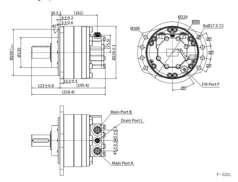
Note: The weight of the connection shown in the figure is 46.8kg.
