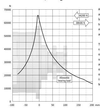
As shown in the figure, when the axial load is 0, the radial allowable load of the output shaft is related to the distance from the flange mounting surface to the load action point.
