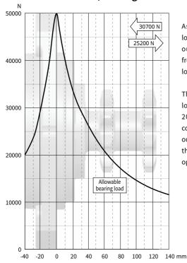
As shown in the figure, when the axial load is 0, the radial allowable load of the output shaft is related to the distance from the flange mounting surface to the load action point.
