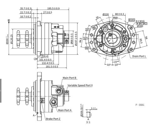
Note: The weight of the connection shown in the figure is 35kg.
