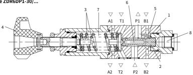
Note: Because there is internal leakage, when sandwich plate pressure reducing valve is used in pairs with sandwich pilot operated check valve , pressure reducing valve must be fixed between the check valve and directional control valve.
