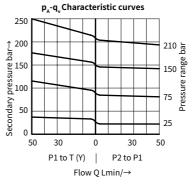
**Note:** if the set pressure is low, the performance curve is within the corresponding pressure level range.
