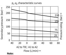
The curve characteristics remain, with low set pressures, the same in relation to the pressure rating.
