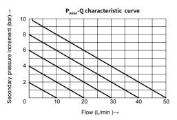
25 bar PA min-Q characteristic curve shows the flow from A1 to A2 in relation to the adjustable min. setting pressure from P2 to P1.
