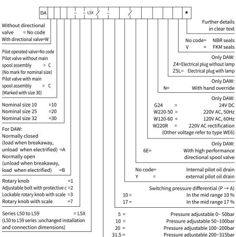
Note: Y (Outer) type is recommended for large pump flow rates and low switching differential pressures (10%).
