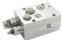
Counterbalance Valve for Telescopes(Boom lift) Flow: Valve 1 ≤ 60 L/min 、 Valve 2 ≤ 150 L/min Pressure: ≤ 350 bar
